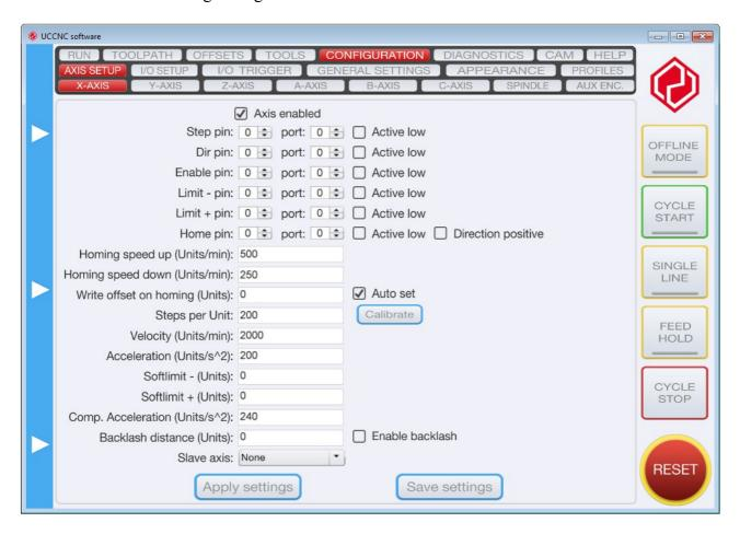
**Step port & pin:** Which is the physical output pin on the UC100 device for the step signal. The signal can be configured active low or active high selecting or unselecting a checkbox next to the control.
