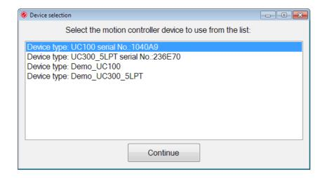
The device selection window lists all the available motion control devices which are actually cunnected to the PC and also it lists the available demo modes to run the software in. The devices
