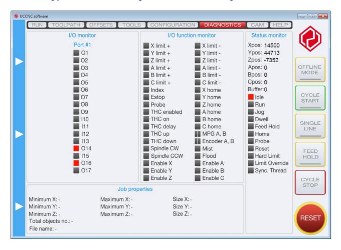
The following printscreen shows the diagnostics screen when running the software with the UC300-5LPT:
