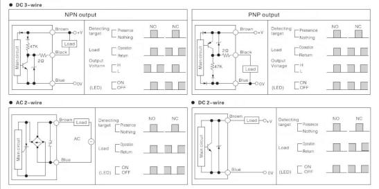
Remark: Be sure to correctly wire the sensor, otherwise may cause the malfunction
